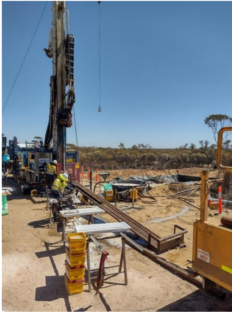
Diamond Drilling in progress at the Boomerang Kaolin Prospect
