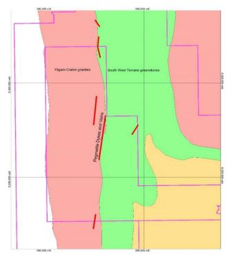
Figure 1 Mapped pegmatites (red) over the 1:100k state interpreted bedrock geology.
