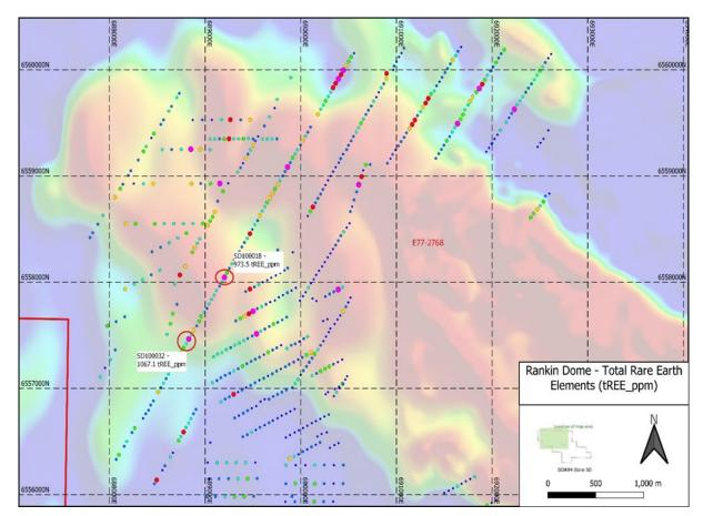
Figure 3: Auger geochemistry results (tREE ppm) over reprocessed regional RTP-TMI\_VD1e magnetics.
