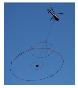
Figure 3: Helicopter with VTEM receiver underneath
