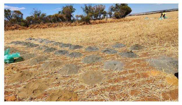
Figure 2: Drill cuttings ready for sampling in an open paddock
