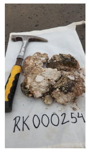
*Figure 13:* Weathered pegmatitic vein from location RK0000254 (54ppm Li and 48ppm Ta).
