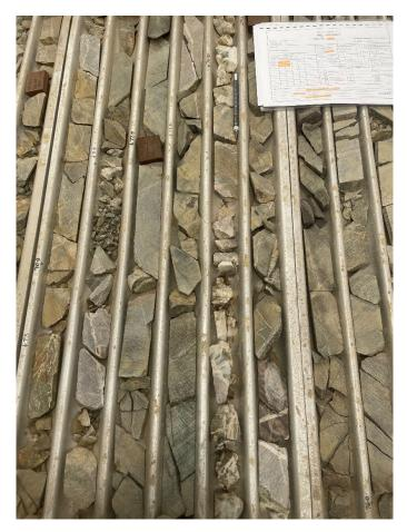
*Figure 2*: Drillhole DDB-1 diamond core tray, zone of pegmatite interest from 73-74m for full suite analysis.
