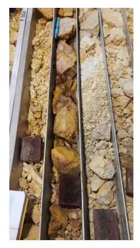
**Figure 3**: DDB-20 diamond drill core with zones of interest for full suite analysis, previous intersection of 1m at 51g/t gold from 39m. (left image is a zoomed in version of right).
