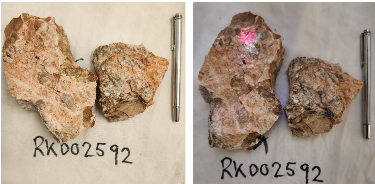
Figure 3: Pegmatite outcrop rock chip RK002592 in natural light on the left and under UV light on the right, noting the pink fluorescence. Pegmatite: Quartz (45%), K-Feldspar (45%), Biotite (10%), no sulphides.
