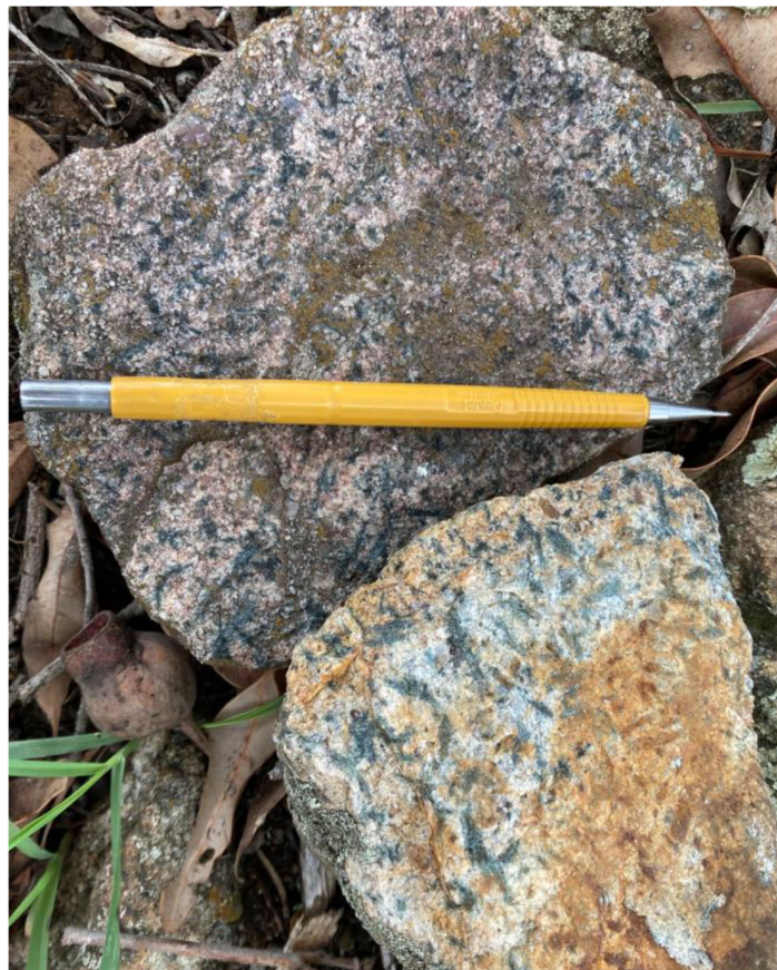
Figure 2: Recent rock chip RK000427 by Kula geologist in the Mustang Prospect with a weathered pegmatite, large green crystals with bladed spodumene and/or tourmaline in a 100% felsic matrix, no sulphides (as expected for this style of mineralisation).
