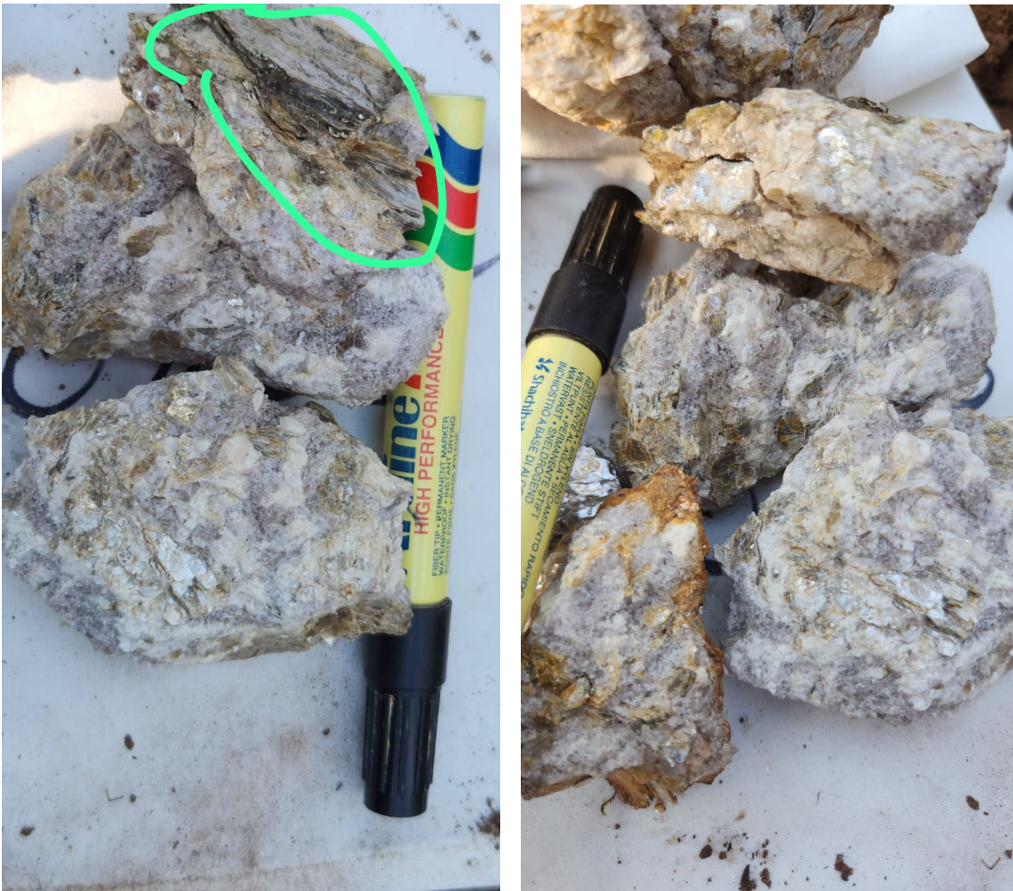
Figure 5: Recent rock chip RK000405 from the Cobra Prospect near a 240ppm lithium rock chip. Pegmatite – large muscovite crystals (>3cm) – purple muscovite purple, grey colour Quartz (45%), K-Feldspar (45%), Biotite (10%), no sulphides (as expected for this style of mineralisation).
