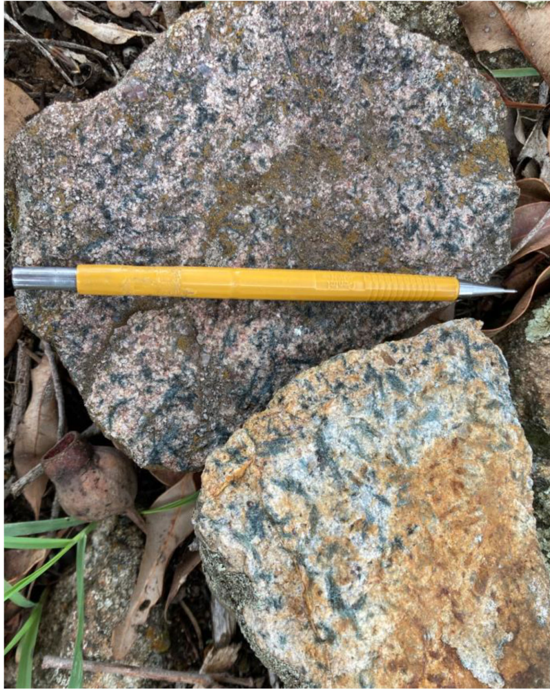
Figure 3: Recent rock chip RK000427 by Kula geologist in the Mustang Lithium Prospect with a weathered pegmatite, large green crystals with bladed spodumene and/or tourmaline in a 100% felsic matrix, no sulphides. (Refer ASX Announcement dated 16 August 2023 – Kirup Lithium Targets – Drilling)
