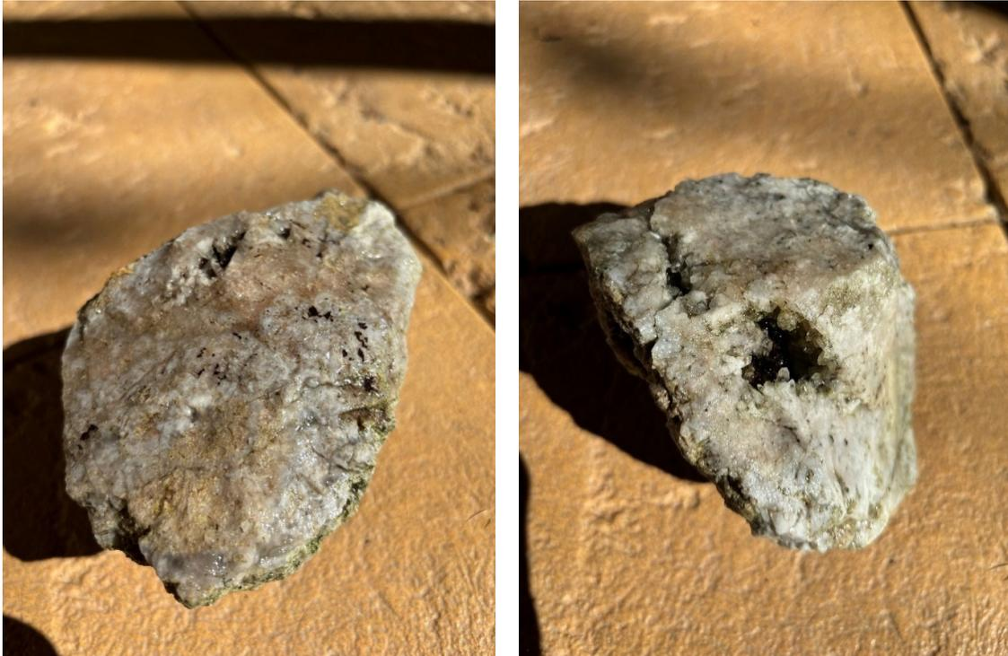
**Figure 3:** Rock chip for the Cobra Prospect, noting the vuggy texture in the quartz host. No visual sulphides are evident in this surface sample, but relic textures are present, and this has not been assayed. (as it is a vector to drilling deeper below surface to the precious metals horizon- ref fig 6).
