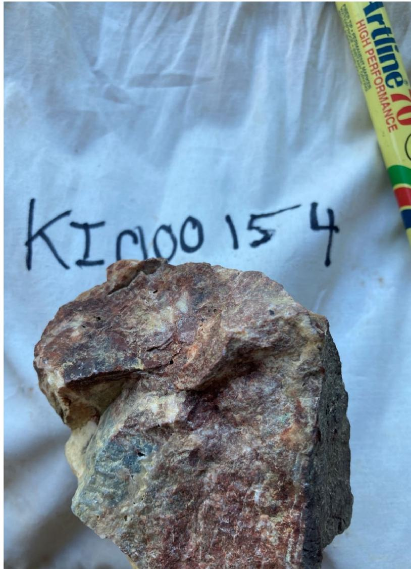
**Figure 7:** Rock chip sample KI000154 with a gold assay of 3.5g/t for the Mustang Prospect, note the vuggy texture in the quartz host. No visual sulphides are evident, but relic textures are present.
