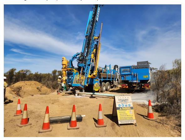
Figure 2: Boomerang Gold Prospect RC drilling.
