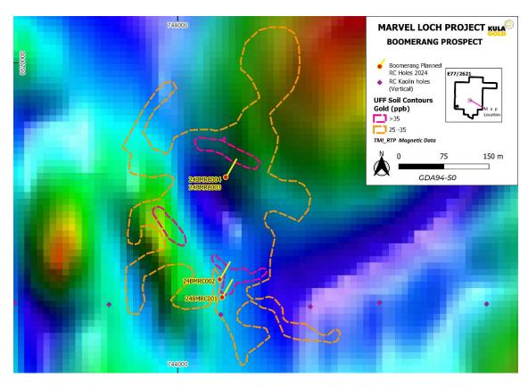
**Figure 3:** Boomerang Gold Prospect with gold UFF soil anomaly and proposed RC drill collars over magnetic TMI\_RTP.
